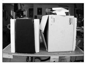
Cut some styrofoam into snug-fitting pieces that fit the interior of the box exactly. I used 2" thick pieces for the front and back of the cabinet, and 1" thick pieces for the top, bottom and sides.
