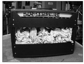
Place a layer of bubble wrap over the speaker and fill the cabinet with crushed newspaper. Pack the container holding the tubes into the newspaper. Reinstall the back panel.
