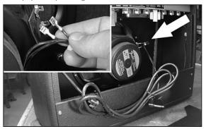
Coil the power cord and tie it with twist-ties so that you can lay it in the bottom of the amp cabinet. Be sure to unplug the speaker leads.
